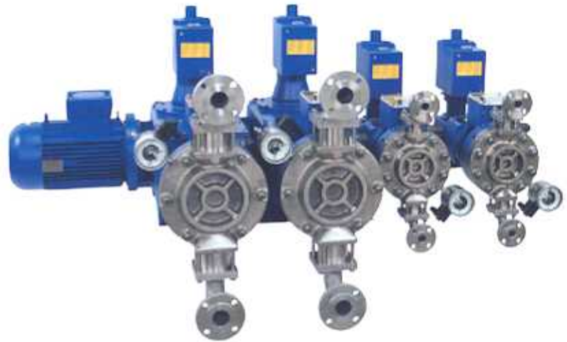
Multiplex metering pump type H4-42 P42 with diaphragm pumpheads and flow rate control via individual electric stroke length adjustment
