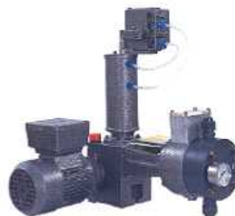
Metering pump type PSI with plastic diaphragm pumphead and flow rate control via pneumatic stroke length adjustment
